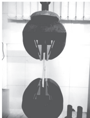
Figure 5: Friction testing in Universal testing Machine
